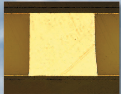
Pure gold filled via cross-section viewed at 100X magnification
